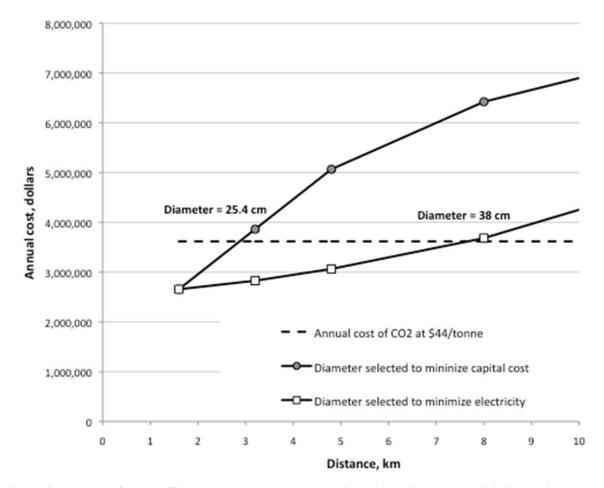
Figure 4. Example of trade-off in annual cost between selecting a pipe diameter to minimize capital cost or to minimize electricity cost for a case in which a coal power plant was the CO<sub>2</sub> source for the 405-ha set of open algae ponds, and high algae productivity was assumed. For this case, 6 parallel pipes were selected.
