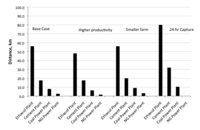
Figure 7. Cost-effective CO<sub>2</sub> transport distances (relative to \$44/tonne CO<sub>2</sub>) for the resources considered under base-case, higher-productivity, smaller-facility, and 24-hr-CO<sub>2</sub>-capture conditions. These results correspond to a configuration that minimizes the electricity cost at the cost of greater capital expense. NG is natural gas.
