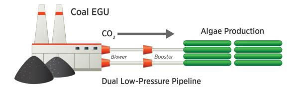
**Figure 1. Illustration of co-location strategy to use CO<sub>2</sub> emissions from a power or process plant.** In this figure, the source is a coal-fired power plant (EGU=electricity-generating unit). The number and size of blowers and pipelines vary with gas volume.
