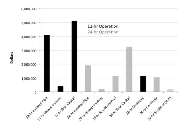
Figure 8. Comparison of costs for 12-hour base-case CO<sub>2</sub> transport with the 24-hr CO<sub>2</sub>-capture case for a coal power plant at an 8-km distance. The difference between sum of the first two bars and the third is the approximate cost for a storage buffer for the gas as it reaches the ponds (see text).
