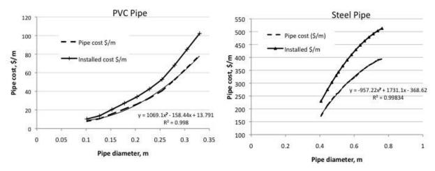
Figure 2. Costs of PVC and steel pipeline based on Peters, et al. [28], and updated to 2014 dollars. Installation factor based on Janna [29].
