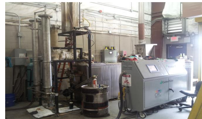
Pilot auger pyrolysis reactor at UTK Center for Renewable Carbon
