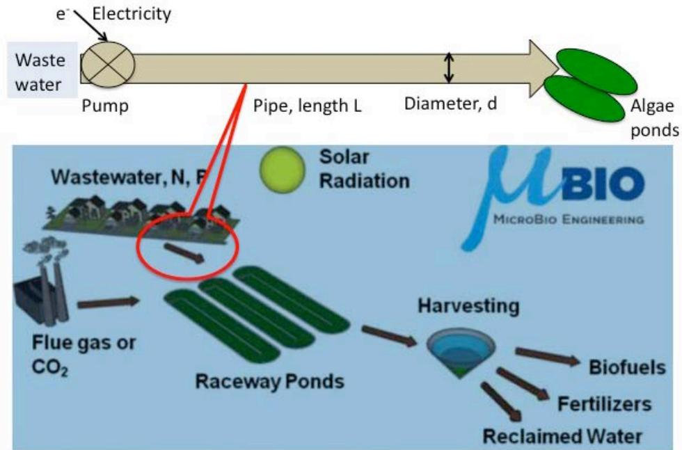
**Figure 1. Simple depiction of a wastewater transport system for an open-pond algae production system, based on a MicroBio Engineering approach [10]. Used with permission from Microbio Engineering, Inc.**
